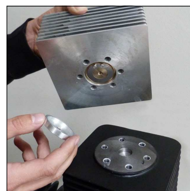
Fig. 2 - Remove lower valve gasket
