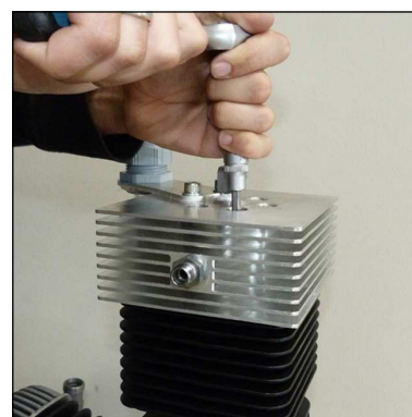
Fig. 1 - Loosen valve head screws
