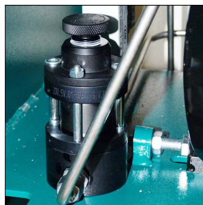
Safety valve 4th stage
