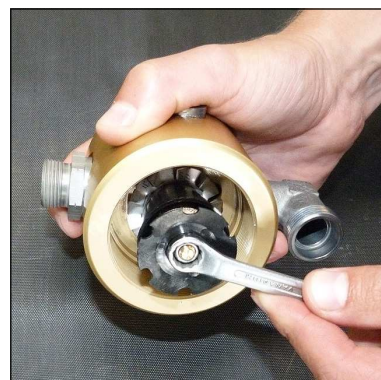
Fig. 2 - Loosen nut at the separator top
