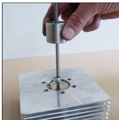
Fig. 3 - Remove inlet and outlet valve
