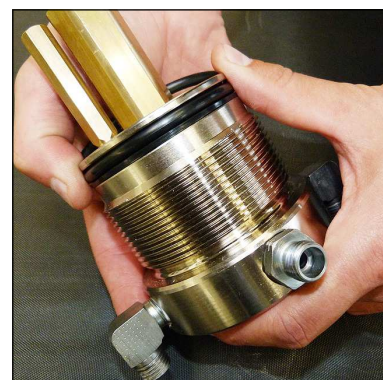
Fig. 4 - Change o-ring and back-up rings
