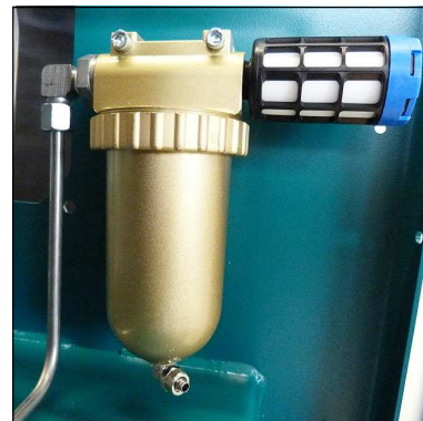
Oil / water separators final stage
