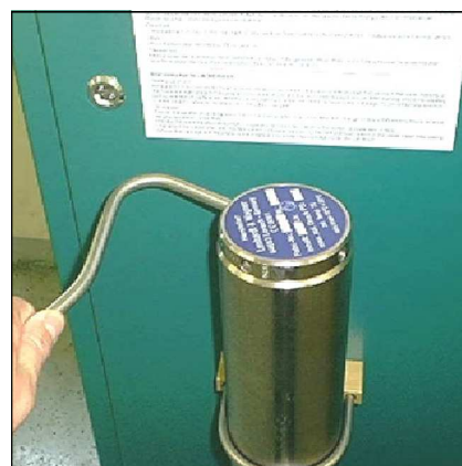
Fig. 1 - Unscrew the filter housing cover.
