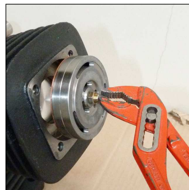
Fig. 2 - Pull out inlet and outlet valve
