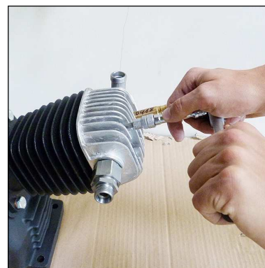
Fig. 1 - Loosen valve head screws
