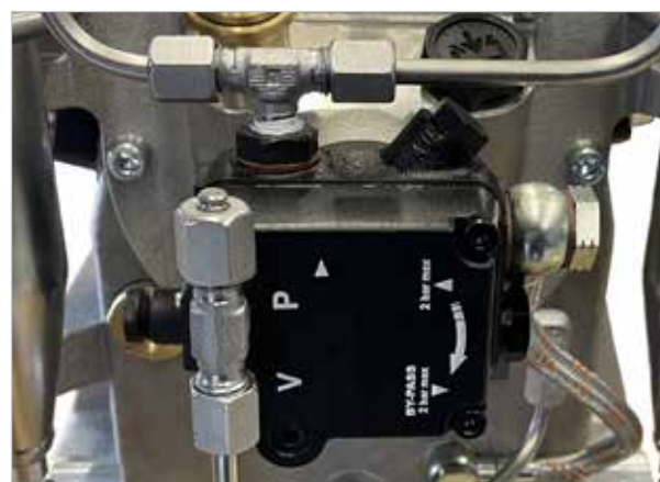
NEW - Adjustable oil pump with oil sieve
