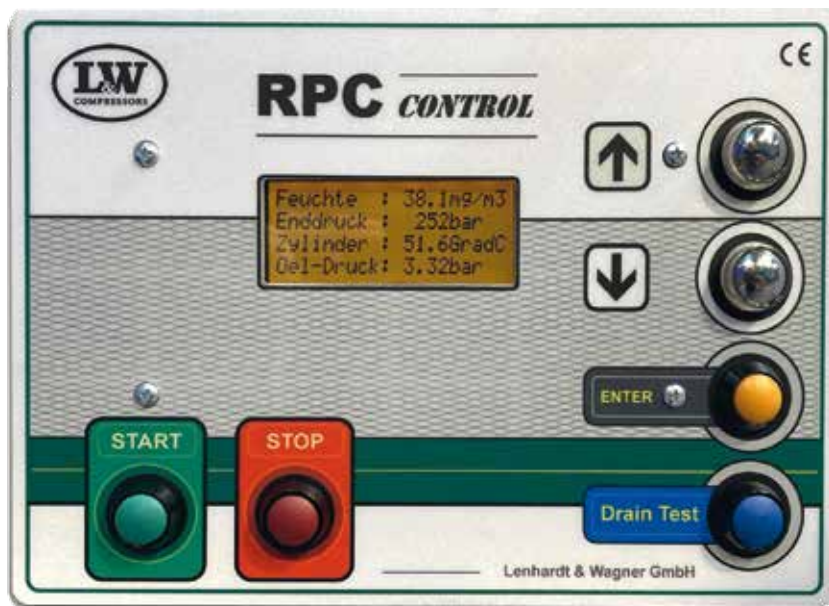
Figure: Standard display at compressor
