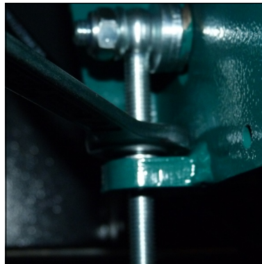
Fig. 3 - Tighten V-belt by the lock nut
