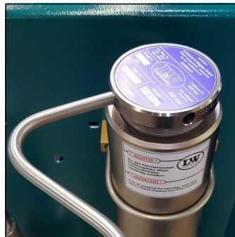
Fig. 2 - Unscrew the filter housing cover.
