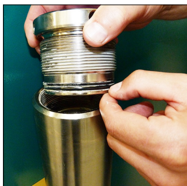
Fig. 2 - Change o-ring and back-up rings
