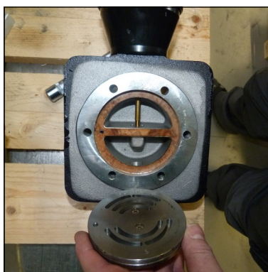
Fig. 2 - Remove in- and outlet valve
