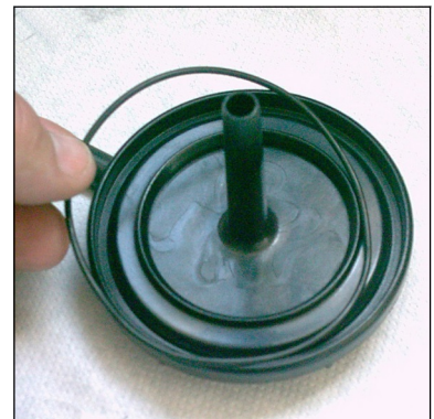
Fig. 3 - Place o-ring into the filter housing
