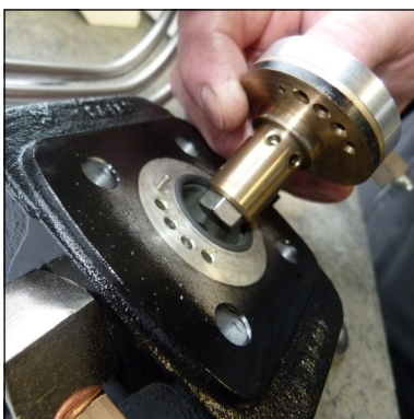
Fig. 1 - Ensure correct valve position (centre pin)
