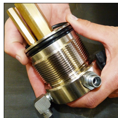
Fig. 4 - Change o-ring and back-up rings
