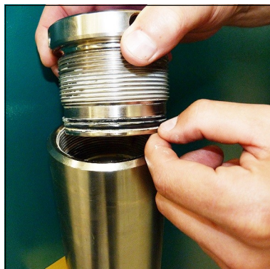
Fig. 2 - Change o-ring and back-up rings
