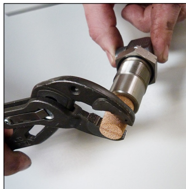
Fig. 3 - Change sinter filter
