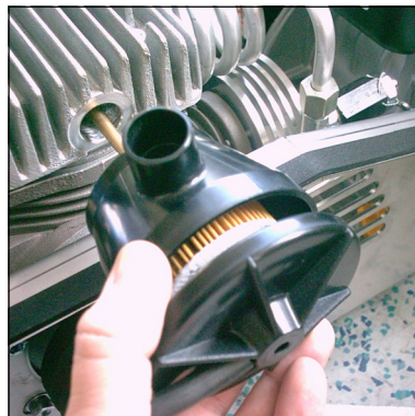
Fig. 2 - Pull out filter housing carefully
