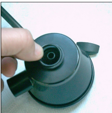
Fig. 4 - Place o-ring into the groove
