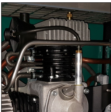
Fig. 1 - Remove spring wire clamps
