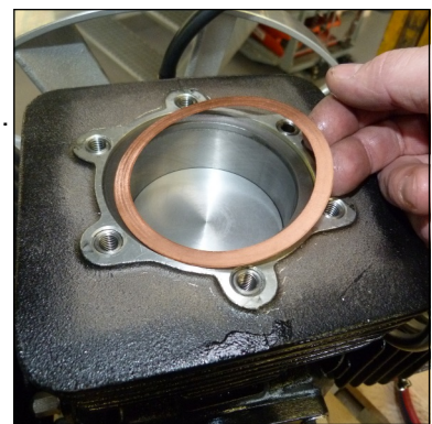
Fig. 1 - Lower valve gasket
