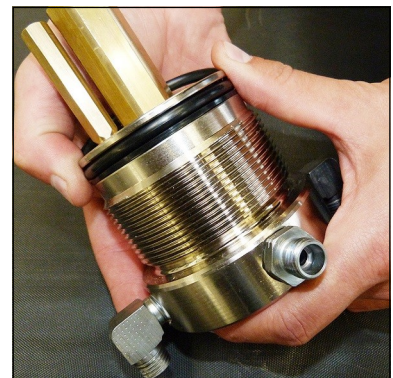
Fig. 4 - Change o-ring and back-up rings
