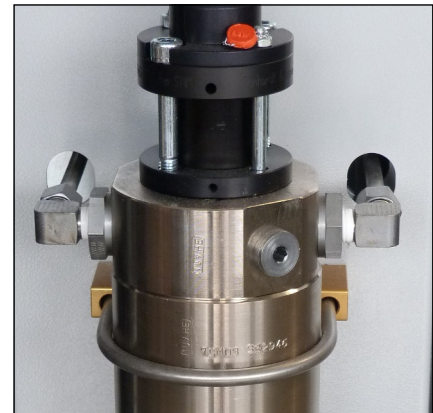
Fig. 1 - Loosen pipe connections and mounting screws
