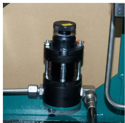
Safety valve 3rd stage
