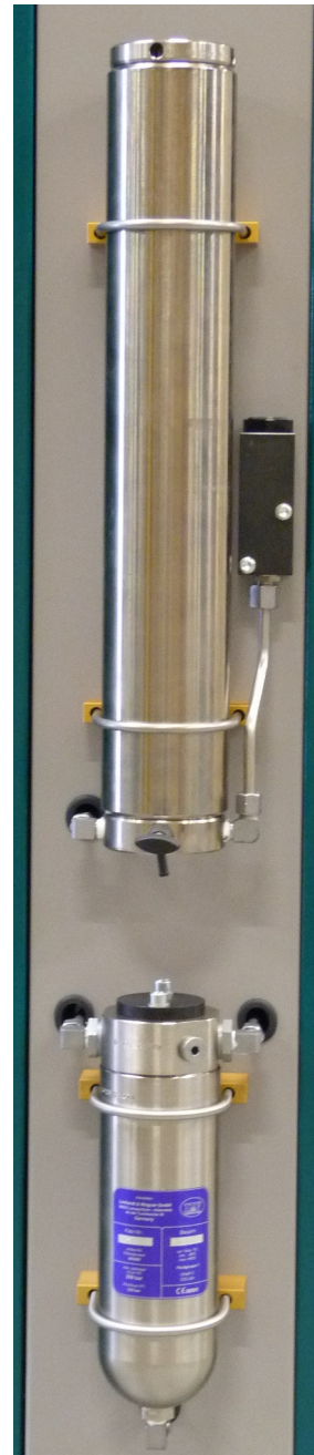
Filterhousing 1.7l (upper), pressure maintaining non return valve and filter unit 0,8l (below)
