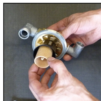
Fig. 3 - Change sinter filter
