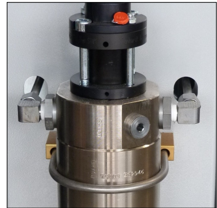
Fig. 1 - Loosen pipe connections and mounting screws
