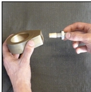
Abb. 8 - Change sinter filter
