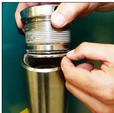
Fig. 2 - Change o-ring and back-up rings
