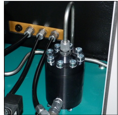
Fig. 1 - Condensate stop valve housing
