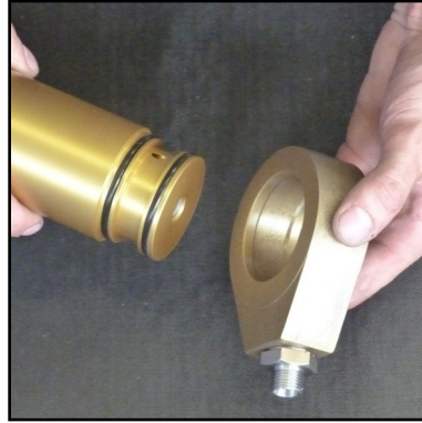
Abb. 5 - Remove the base ring
