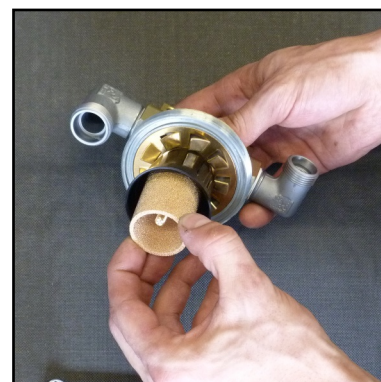
Fig. 3 - Change sinter filter
