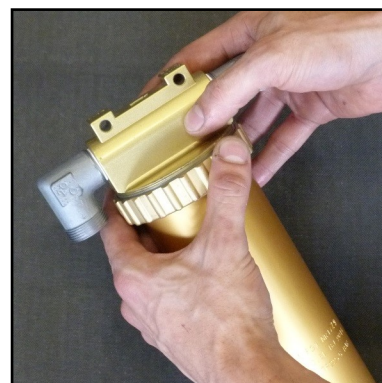
Fig. 1 - Open ring nut and remove separator top
