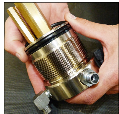
Fig. 4 - Change o-ring and back-up rings
