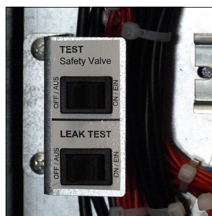
Leak test switch (down)
