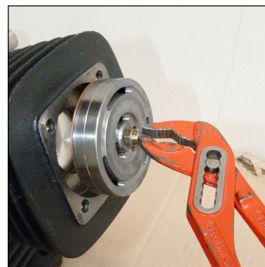
Fig. 2 - Pull out inlet and outlet valve
