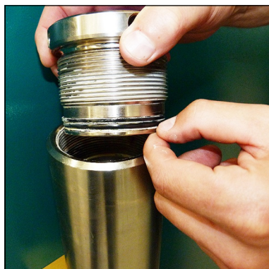
Fig. 2 - Change o-ring and back-up rings
