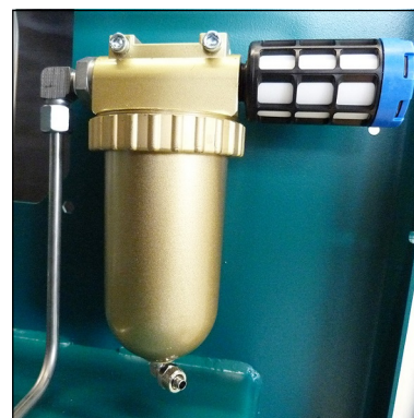
Oil / water separators final stage
