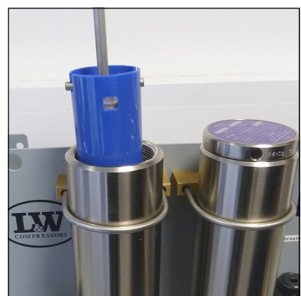
Fig. 3 - Pull the cartridge out of the housing
