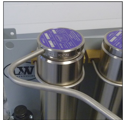
Fig. 1 - Unscrew the filter housing cover
